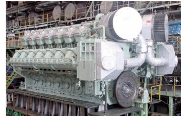
DU-S.E.M.T.Pielstick 14PC4.2BV 18,550kW at 430min -1
