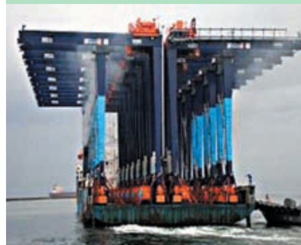
Fifteen RTGs are on a vessel for transportation
