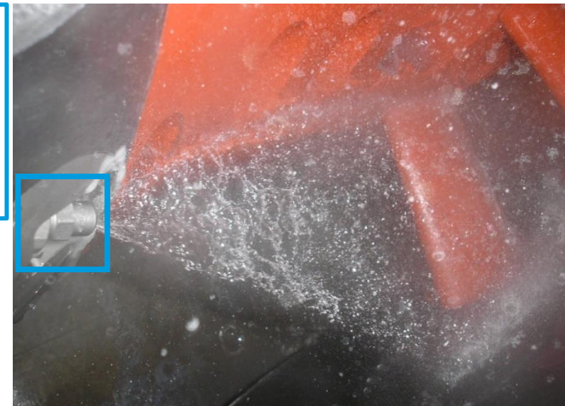
Water Spray Nozzle for WET type TRT
