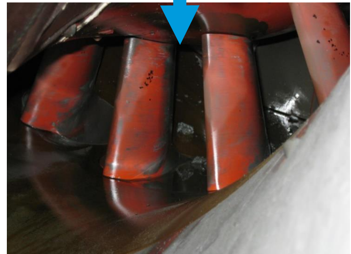
Dust Accumulation on 1 st Stator Blade
