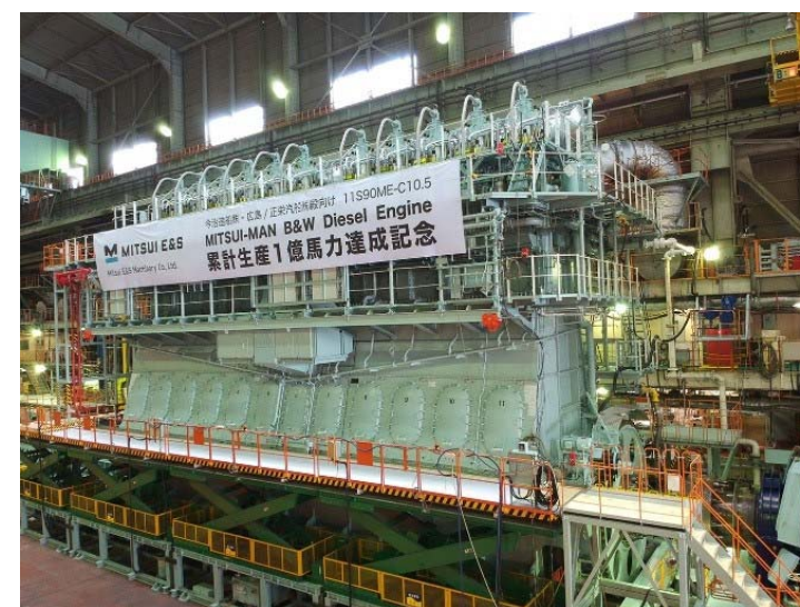
Machine of 100M horsepower(11S90ME-C10.5)
