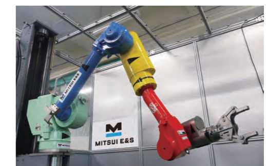
A manipulator for HD06 decommissioning
