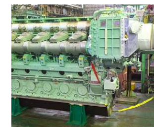
S.E.M.T. 12PC2.6BV medium-speed four-stroke engine
