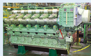
S.E.M.T. 12PC2.6BV medium-speed four-stroke engine
