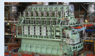
MAN B&W 8S70ME-C8.2-GI LNG-fueled diesel engine
