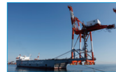
The salvage barge with a fork : “Tenyu”, built by Mitsui E&S Shipbuilding (Tamano Shipyard)
