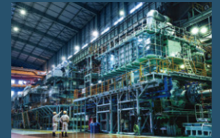
Methanol-burning electronically-controlled gas injection diesel engine (ME-LGI)
