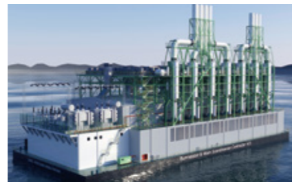
Gas power generation barge
