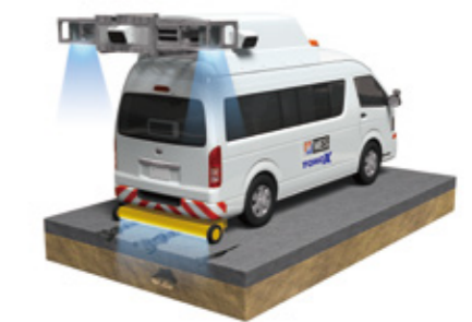
Radar inspection system for road maintenance
