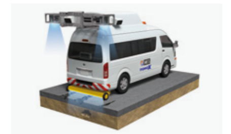
Vehicle for radar inspection
