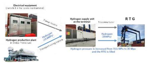
(3) Cargo handling operations using cargo handling machinery (including hydrogen filling for cargo handling machinery)
