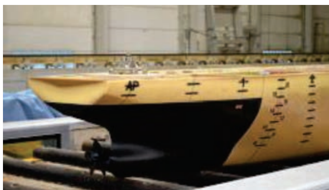
写真1 模型船 LJBC (船尾) Model Ship of LJBC (Aft)
