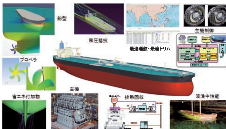
図1 CO 2 排出量 30% 削減船の要素技術の概要 Outline of Technology Elements of the Ship with Reduced CO 2 Emission by 30%
