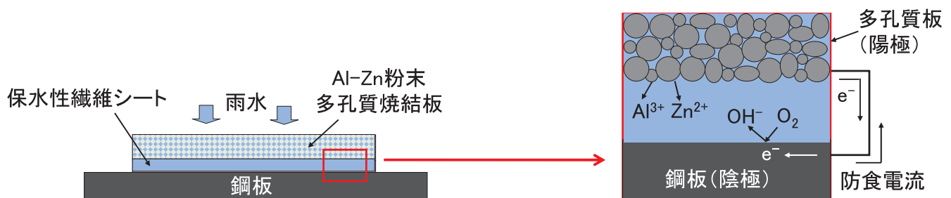
図1 防食メカニズムの概念 Conceptual Model of Mechanism of Corrosion Protection
