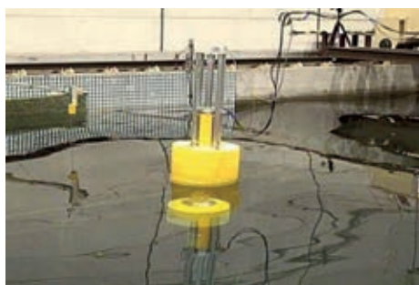
写真3 同調制御の実験装置(潮流水槽) Experimental Device of Resonance Control(Current Water Tank)
