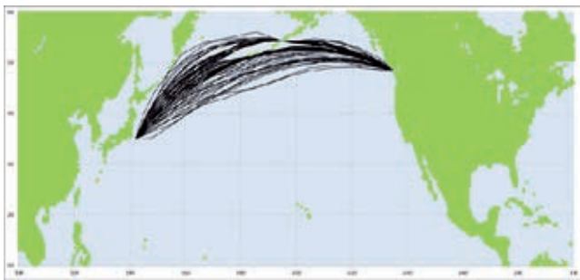
図7 計算航路例(日本近海～シアトル，1月～3月) Example of Navigation Route between JAPAN and SEATTLE from January to March
