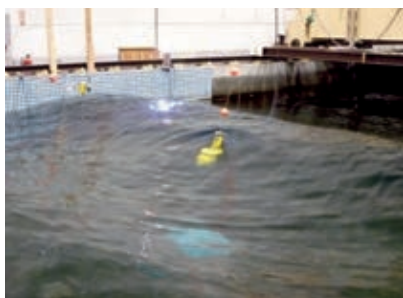
写真5 荒天時のPB-MESの挙動 Behavior of PB-MES in Survival Condition
