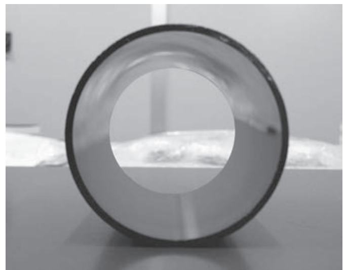
写真1 パイプ内面への DLC 成膜 Example of DLC Inner Coating by PBIID
