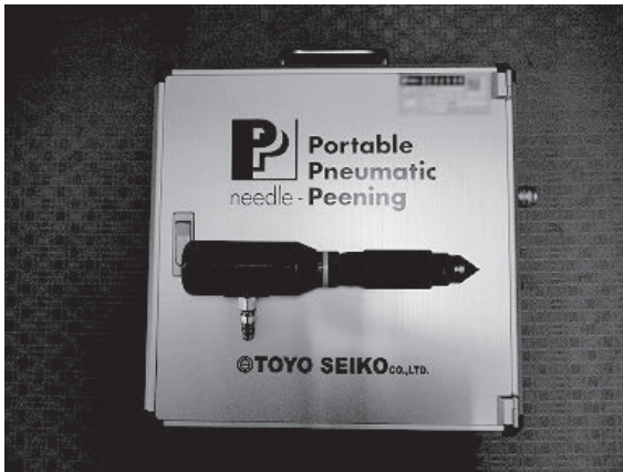
写真2 PPP 装置 Appearance of Portable Pneumatic Needle-Peening
