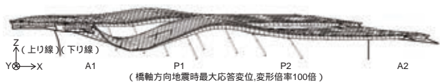
図5 現橋の動的解析変形図 Deformed Drawing in Dynamic Analysis of Current Bridge
